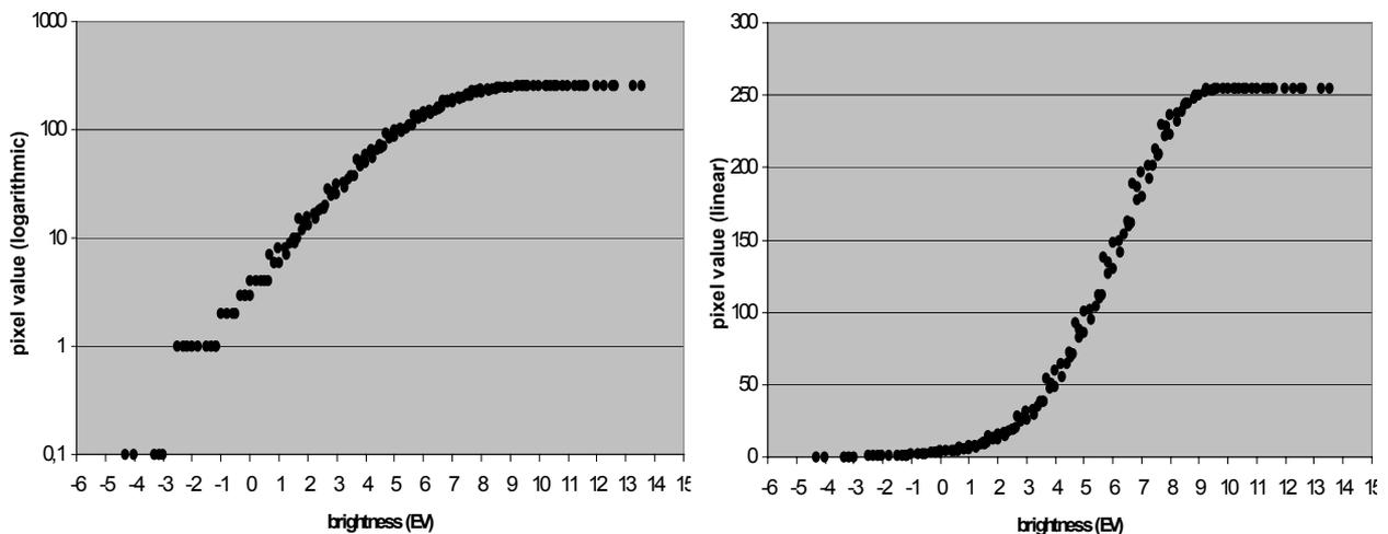
Fig.2: Transmission function for camera JPG (Canon EOS 20D)
